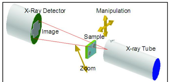
*In general, for off-line 2D x-ray inspection systems, x-rays pass through a sample and are collected on a detector, with magnification possible.*
