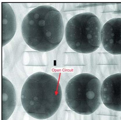
*An off-line x-ray inspection system was used for an angled view (left image) and a close-up view (right image), where an open-circuit failure is visible to a human operator. Such a system offers the control and advantage of enabling investigation of potential failure sites.*
