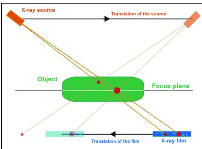
*Basic principle of laminography. Features in the focus plane are always projected on the same position of the detector. Features outside this plane are blurred.*
